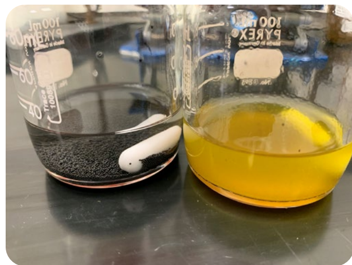
Figure 1. Carboxen® 564 (left) and Silica-Thiol (right) in methanol after a [Rh(COD)Cl] 2 scavenging experiment. The discoloration observed with the Silica-Thiol treated solution is the result of the particles suspended in the solution. Carboxen® 564 quickly settles, as can be seen by the black layer under the stir bar.
