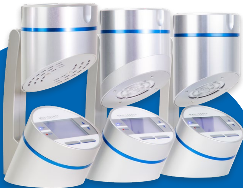
left to right: MAS-100 NT ® , MAS-100 NT ® with filter mounting kit and MAS-100 NT ® with Filter
