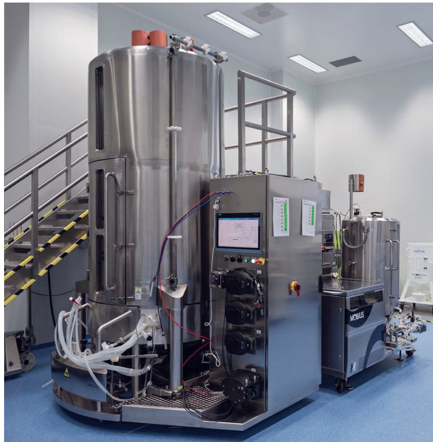
Upstream suite in a mAb manufacturing plant. A major component of a virus safety strategy is preventing viruses from entering the upstream process.
