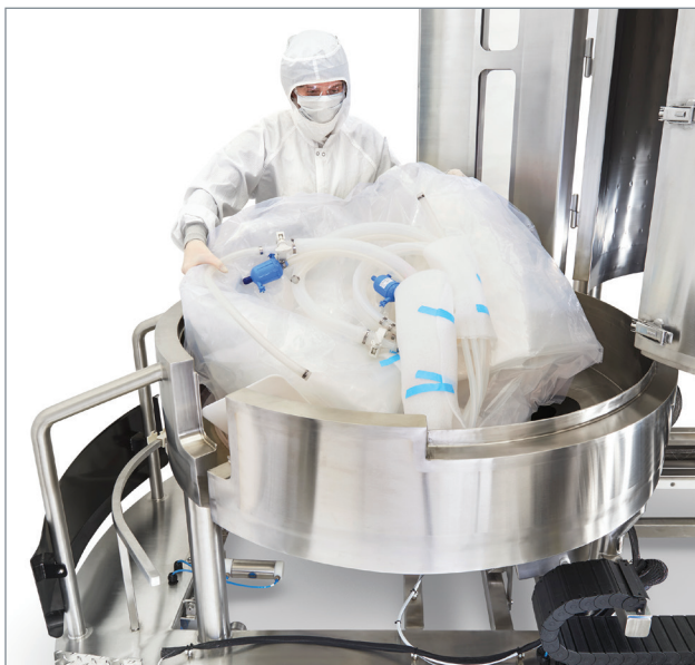
Operator installing a single-use bag in a Mobius® 2000 L single-use bioreactor.
