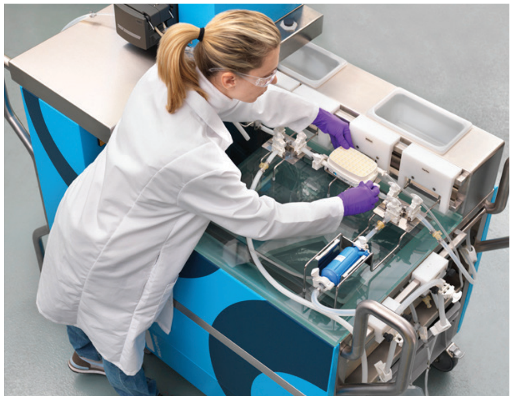
An operator setting up a virus filtration step. Virus filtration removes both enveloped and non-enveloped viruses.
