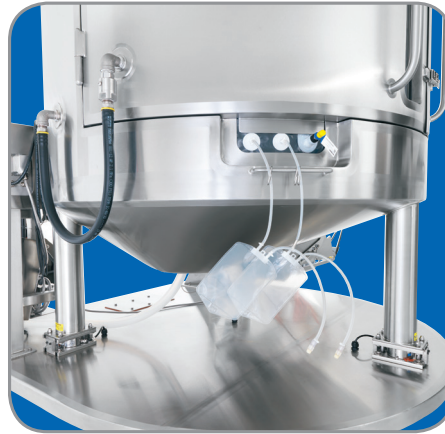
Figure 5. Needle-free sample ports with sample bags and Hamilton OneFerm pH Sensor
