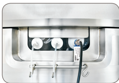
Figure 3. Needle-free sample ports and Hamilton OneFerm pH Sensor on Mobius® MIX 2000 bag
