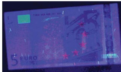
Figure 3. (top) Luminescence of blue ( \text{Eu}^{2+} ), green ( \text{Tb}^{3+} ) and red ( \text{Eu}^{3+} ) phosphors for (compact) fluorescent tubes under 254 nm UV irradiation. The white luminescence is obtained for a mixture of the blue, green and red phosphors. (bottom) Euro banknote under 360 nm UV irradiation. The red, green and blue luminescence from the stars and fibers is generated by \text{Eu}^{2+} (blue and green) and \text{Eu}^{3+} (red).
