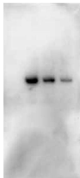
High background and dark edges caused by insufficient washing of the blot. Can be alleviated by additional or/and longer washes or a high salt wash (Protocol 3.4, page 41.)
