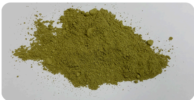
Figure 2. Hemp Buds “Finola” after Grinding in a Cryo Ball Mill. Resulting Particle Size <100 µm.
