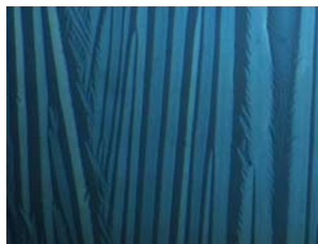
Figure 5. Micrograph of a polymer/TIPS pentacene blended film formed by dip-coating. Note the morphology of the TIPS pentacene crystals is similar to that seen in non-blended films ( Figure 4 ).
